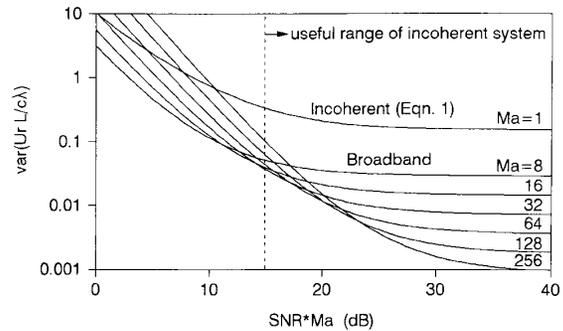
Fig. 1. Cramér-Rao lower bound on velocity variance, comparing two-pulse broad-band systems of various code lengths with an incoherent system of the same range cell size and pulse length (half the total transmission length).
