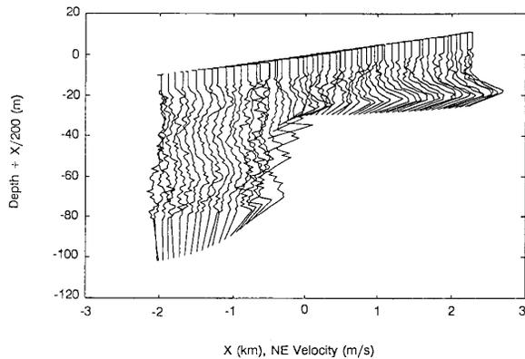
Fig. 5. Stack plot (waterfall plot) of the cross-sill velocity component at slack tide. Profile top and bottom ends have been extrapolated (see text).
