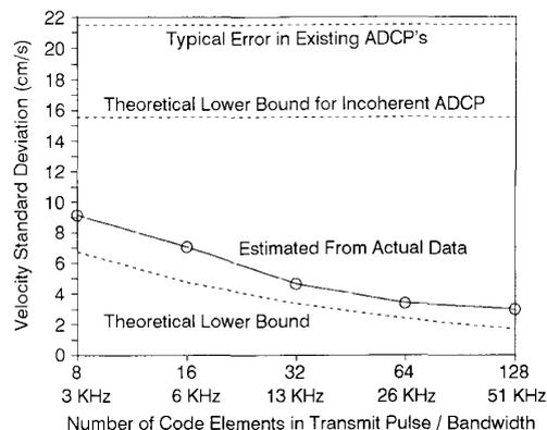
Fig. 2. Radial velocity error as a function of system bandwidth.
