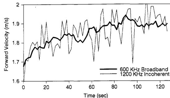
Fig. 4. Comparison of broad-band and incoherent instruments for 1-m (vertical) range cell at 5-m vertical range.
