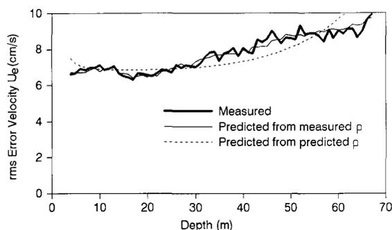
Fig. 3. Measured versus predicted error velocity. Average is over 512 pings.
